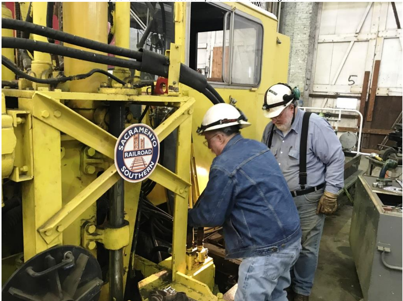
Mike H. and Frank get straps around the kicker's hydraulic cylinder
