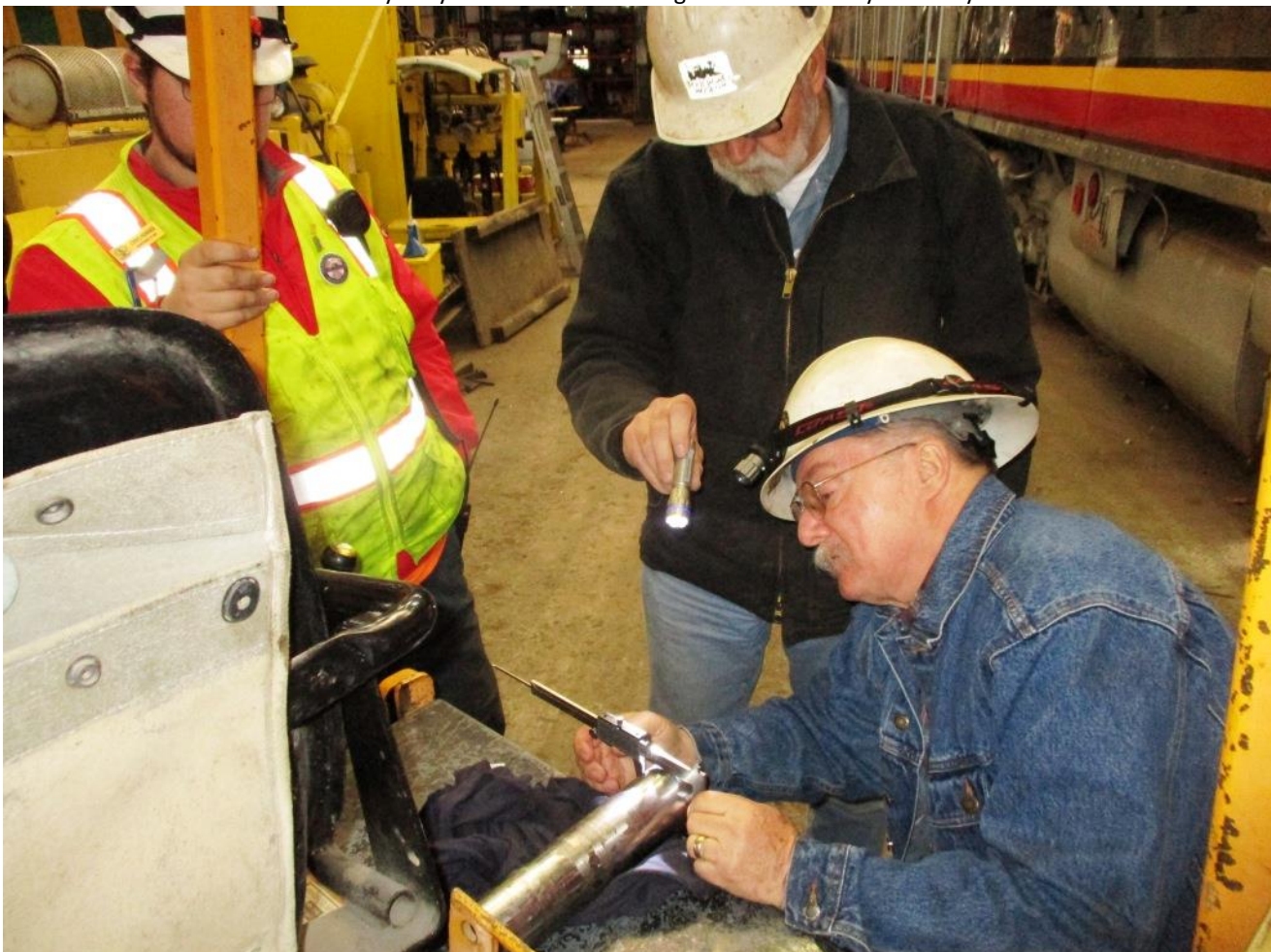
Mike H. uses calipers to measure the diameter of the connecting pin
